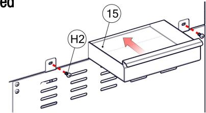
Align mounting holes of grilling chamber with cabinet slots. Attach cabinet and grill head using 2x M6 Phillips Screws (H2) per side. Tilt, then slide 2x Grease Trays (#15) into place.
