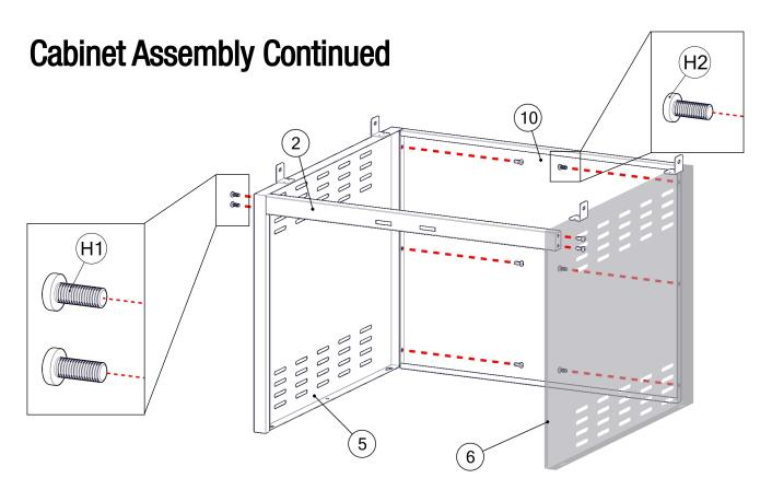
Assemble cabinet sides and back using 6x M6 Phillips Screws (H2).
