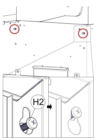
Thread 2x M6 Phillips Screws (H2) into the outer top shelf mounting holes as shown. Leave loose so that shelf keyholes can fit over.
