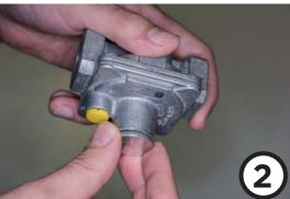
Unscrew the cap to access the regulator adjustment.
