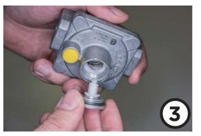
The plastic adapter should be turned upside down depending on the type of gas supply.
